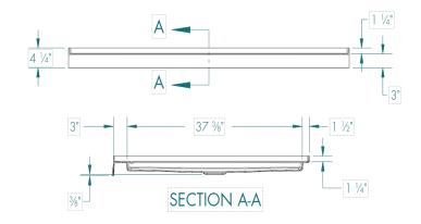
Dimensional Tolerance  $\pm 3/8$ ". Dimensions needed for site preparation should be measured from the unit. Manufacturer assumes no responsibility for preparatory work.
