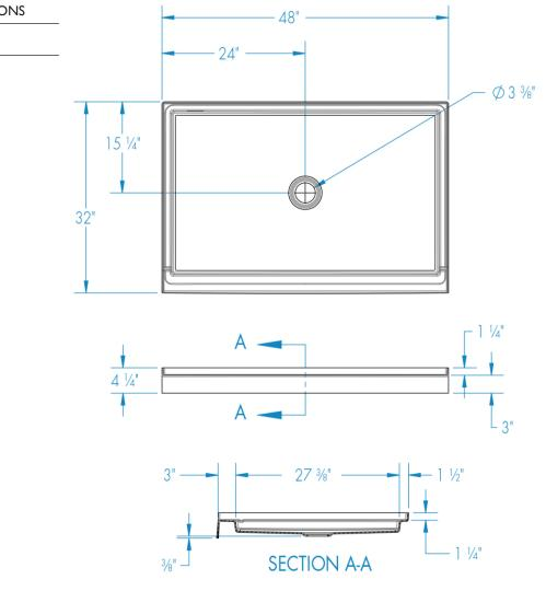
Dimensional Tolerance  $\pm 3/8''$ . Dimensions needed for site preparation should be measured from the unit. Manufacturer assumes no responsibility for preparatory work.
