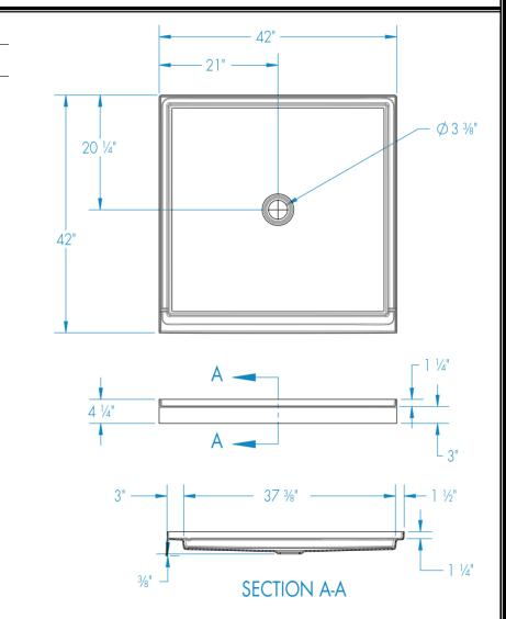
Dimensional Tolerance  $\pm 3/8''$ . Dimensions needed for site preparation should be measured from the unit. Manufacturer assumes no responsibility for preparatory work.
