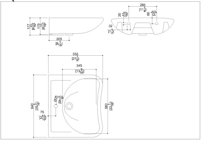
Ergonomic sink with elbow rests made of vitreous china
