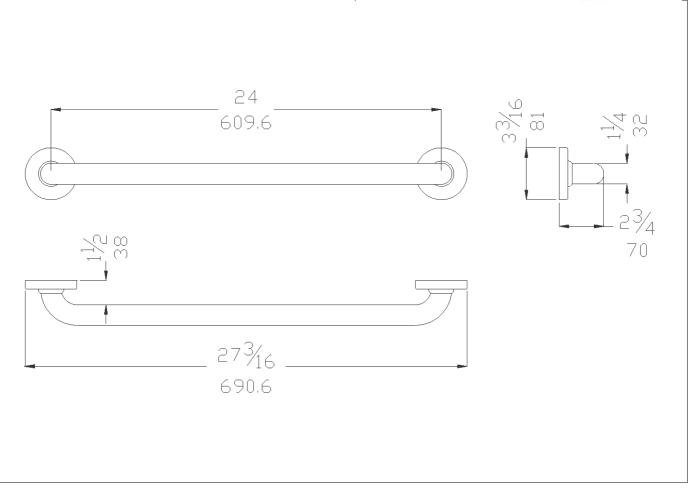
24" Antimicrobial vinyl coated grab bar. No maintenance 3mm thick antimicrobial vinyl coating. Concealed ABS 4-hole flange plate.
