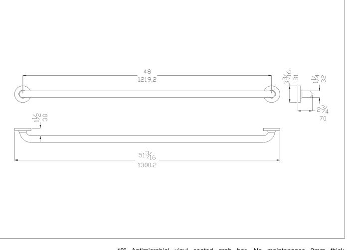
48" Antimicrobial vinyl coated grab bar. No maintenance 3mm thick antimicrobial vinyl coating. Concealed ABS 4-hole flange plate.
