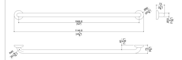
42" straight grab bar, zinc-plated steel pipe, coated with 3mm anti-microbial vinyl, 11-hole concealed mounting flange.
