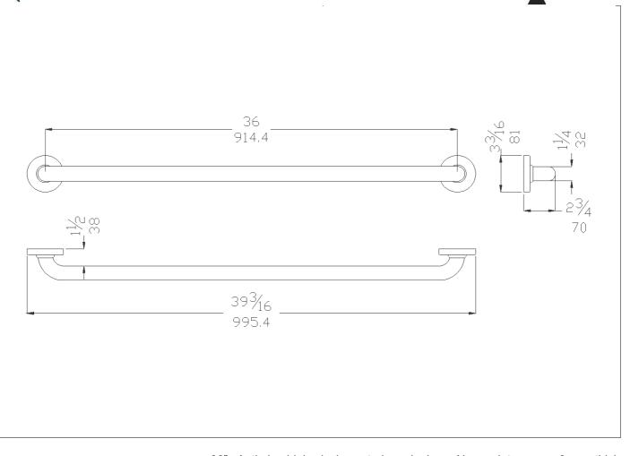
36" Antimicrobial vinyl coated grab bar. No maintenance 3mm thick antimicrobial vinyl coating. Concealed ABS 4-hole flange plate.
