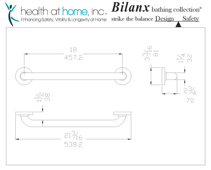
18" Antimicrobial vinyl coated grab bar. No maintenance 3mm thick antimicrobial vinyl coating. Concealed ABS 4-hole flange plate.
