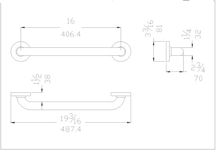
16" Antimicrobial vinyl coated grab bar. No maintenance 3mm thick antimicrobial vinyl coating. Concealed ABS 4-hole flange plate.
