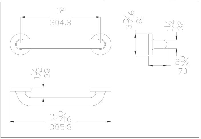
12" Antimicrobial vinyl coated grab bar. No maintenance 3mm thick antimicrobial vinyl coating. Concealed ABS 4-hole flange plate.
