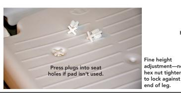
Fine height adjustment—note hex nut tightened to lock against end of leg.
