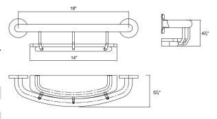
Easy to mount flange! Welded, 3" round, 5 hole flange with concealed cover.
