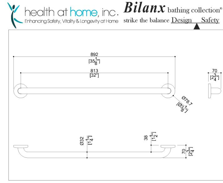
32" Center on center stainless steel grab bar with concealed flange plates. 1.25" diameter, 1.2mm wall thickness, 304 stainless steel.
