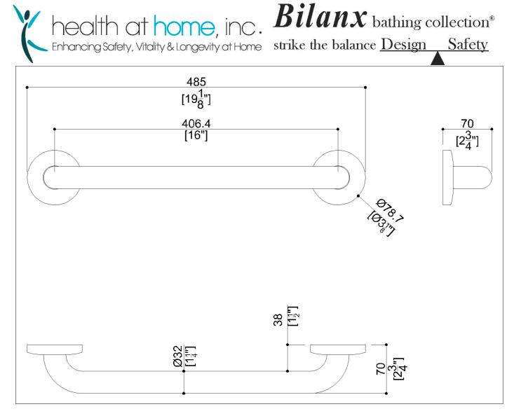
16" Center on center stainless steel grab bar with concealed flange plates. 1.25" diameter, 1.2mm wall thickness, 304 stainless steel.
