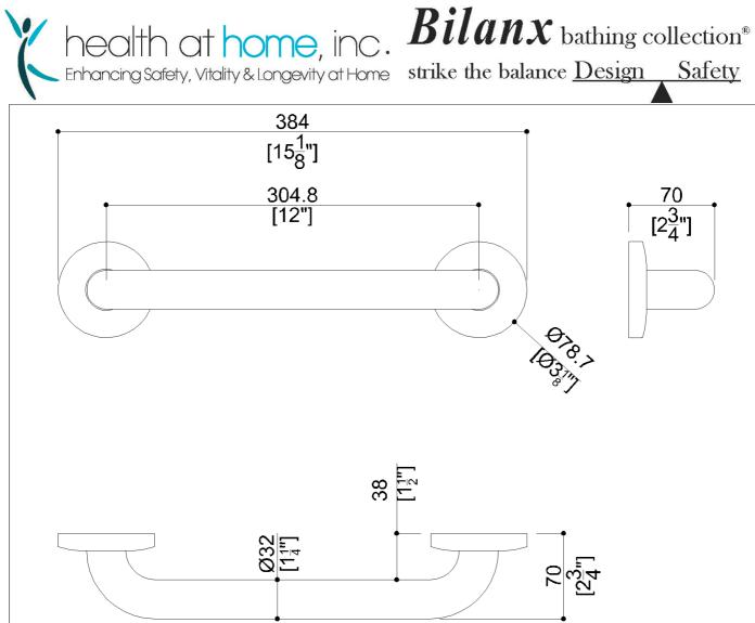
12" Center on center stainless steel grab bar with concealed flange plates. 1.25" diameter, 1.2mm wall thickness, 304 stainless steel.
